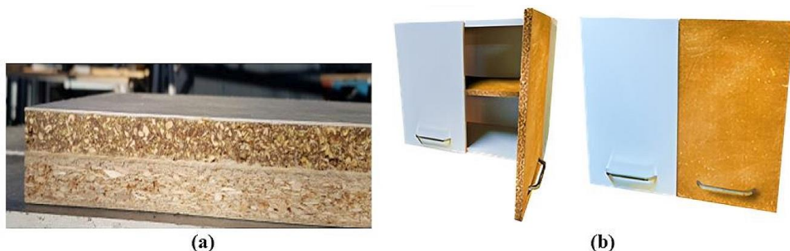
Figure 5. Side view of melamine-coated MDF and, respectively, the sandwich composite (a); the wardrobe with a door and a shelf made of the sandwich composite (b)
